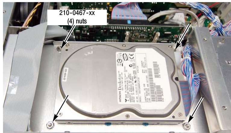
Figure 3: Removing the nuts securing the hard drive mounting plate
