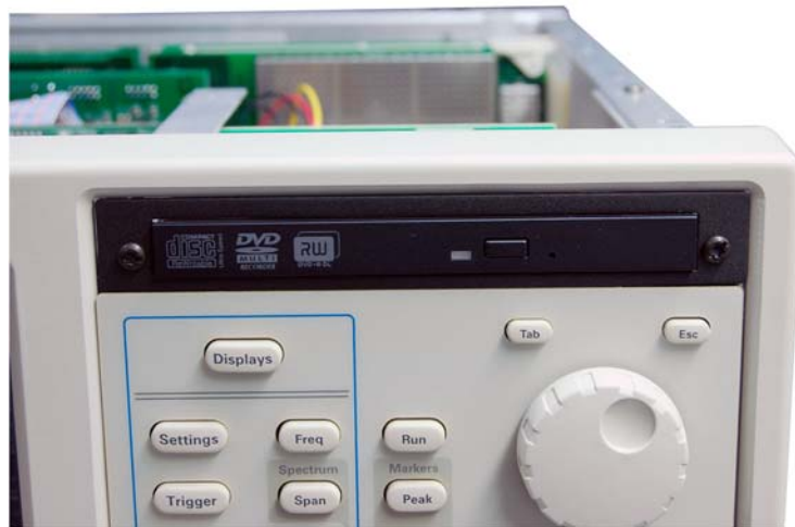
Figure 16: Installed DVD trim ring
