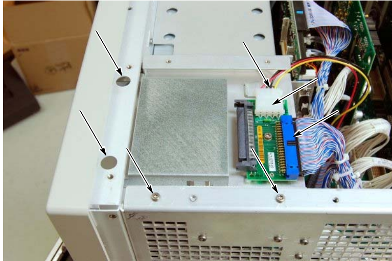
Figure 13: Removing cables from the IDE adapter board and removing the screws that secure assembly
